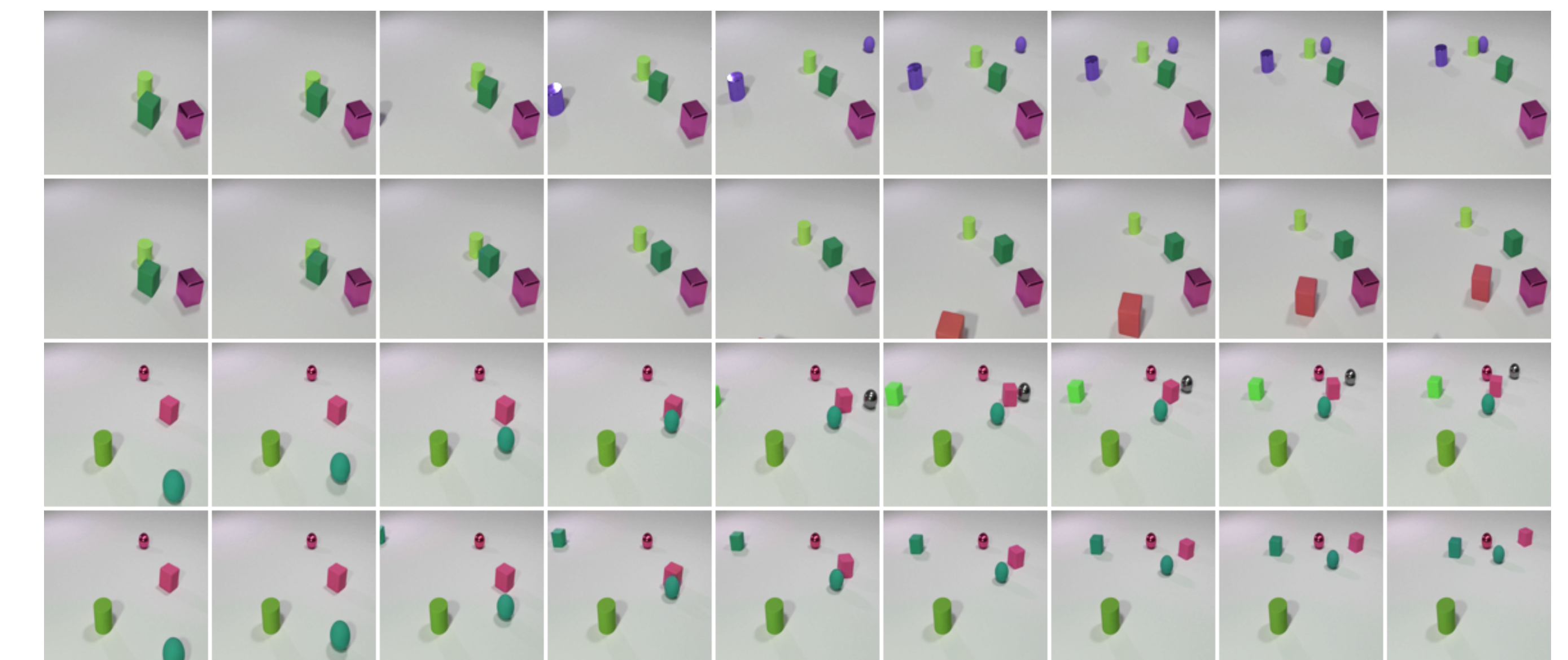
Figure 2. Top row: Real trajectory. Second row: Generated trajectory. A new, red cube enters the scene. Third row: Real trajectory. Fourth row: Generated trajectory. A new green cube enters the scene, and collision physics is respected (green ball hits red cube).
